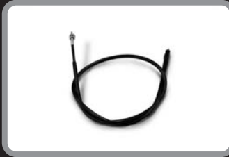
Long speedometer cable For ZOOMER & BITE ZOOMER 300mm 09-01-0110 BITE 40mm 09-01-0111
